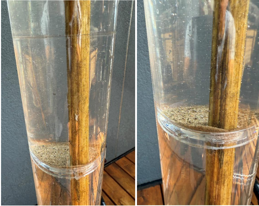
FIGURE 34 – MUDSHARK FLOW LOOP TESTING WITH SUCCESSFUL BUSTING UP OF A HIGH-CONCENTRATION SOLIDS SLUG AND CAPTURING OF THE SOLIDS INSIDE THE CUPS
