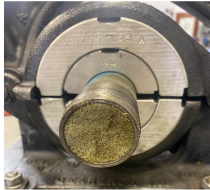
FIGURE 1 – PUMP FAILURE WITH BARREL, SOLIDS PACKED BELOW PLUNGER
