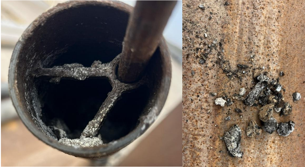
FIGURE 43 – SOLIDS SEPARATED AND COLLECTED/CONTAINED INSIDE A MUDSHARK CUP
