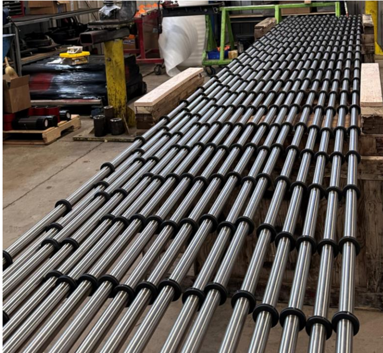
FIGURE 22 – SHARKGUT MANUFACTURING SHOWING 19 WEIRS PER 20-FOOT-LONG MUD JOINT INSERT
