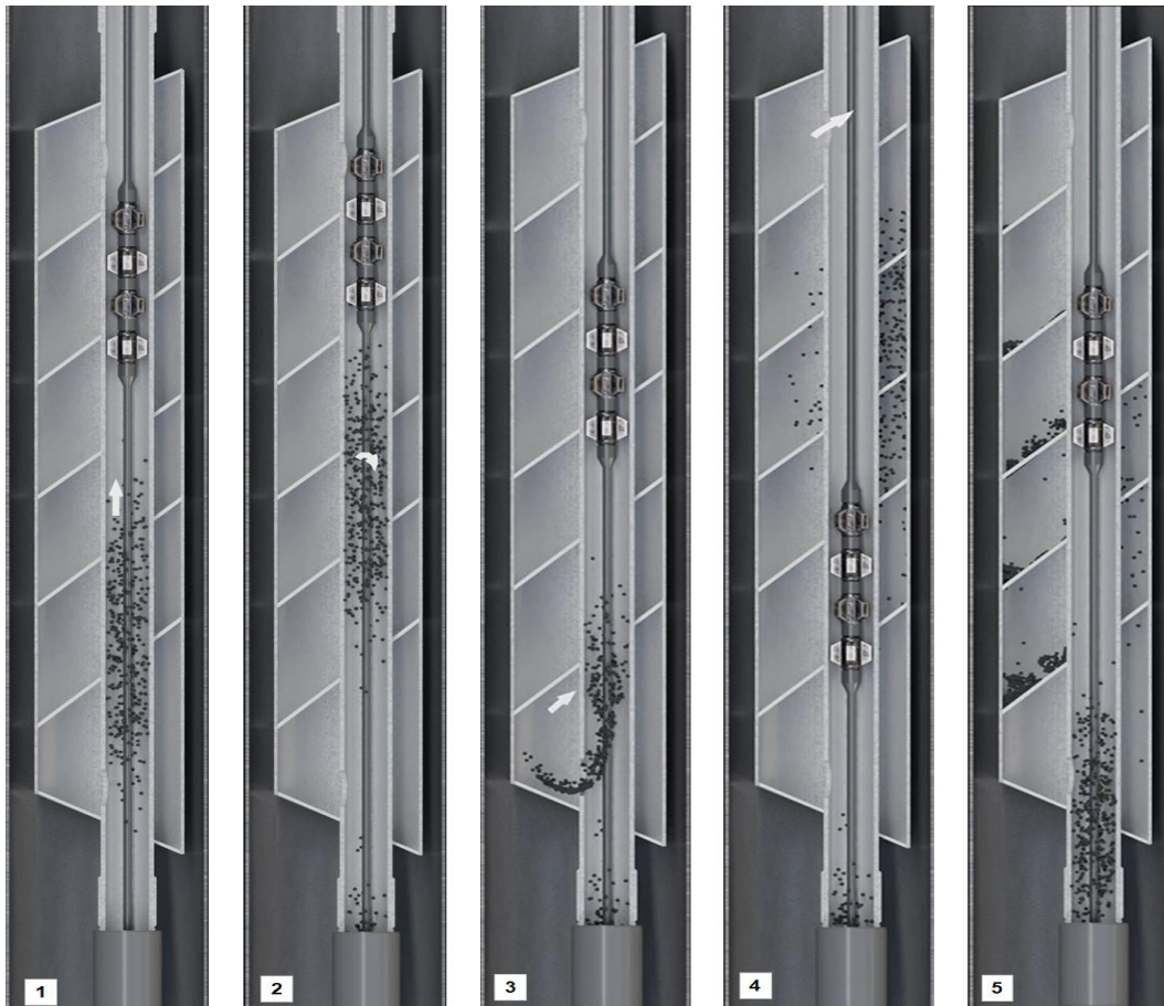
FIGURE 36 – SANDSHARK’S UNIQUE PUMP SOLIDS FALLBACK PROTECTION SOLUTION WITH SEPARATION AND CONTAINMENT ABOVE THE PUMP
