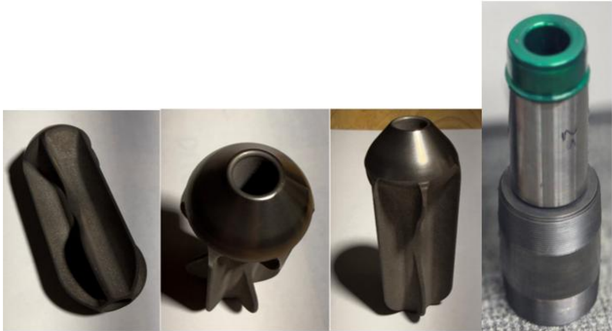
FIGURE 30 – 3D METAL PRINTED PORTED HAMMERHEAD REVERSE FLOW PROTECTION VALVE FOR CONTROLLING PUMP UNSEATING RISKS
